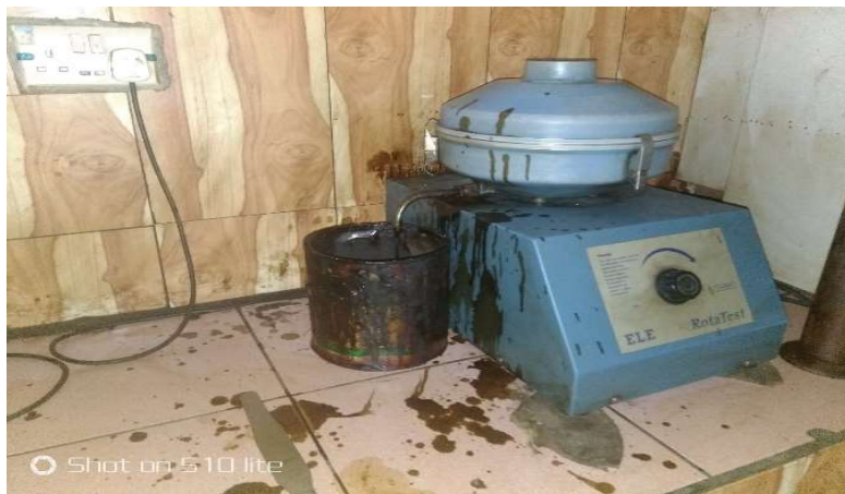
Figure 4: Bitumen Extraction from samples
