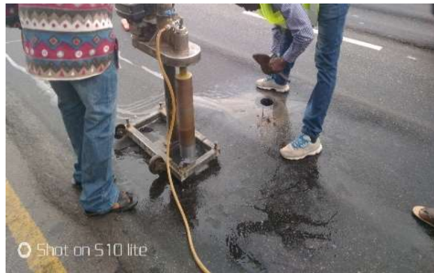
Figure 3: Asphaltic sample coring along Abuja-Lokoja road
